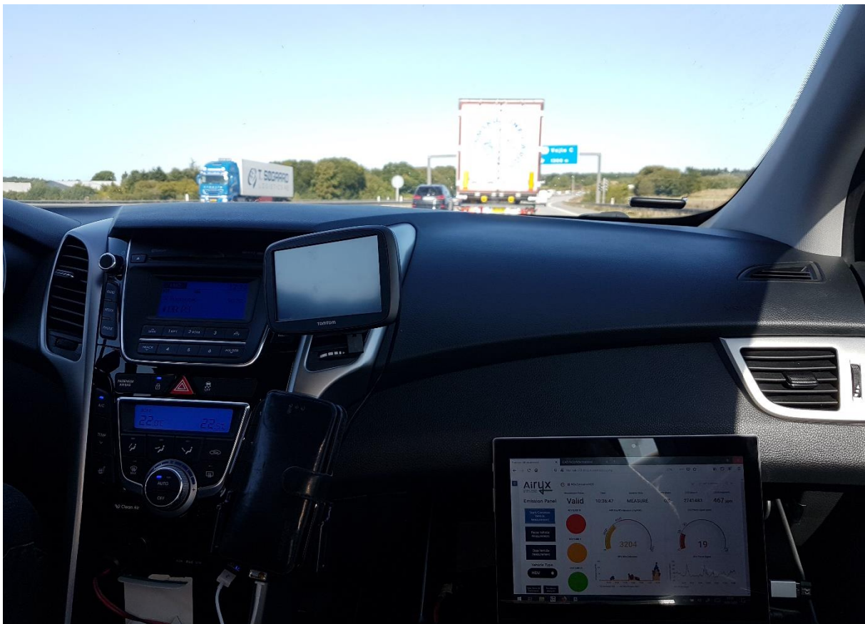
Figure 4: Display installation in the cockpit. A tablet is used as display of the real time data connected via WiFi to the ICAD instrument. It allows operation and visualisation.
