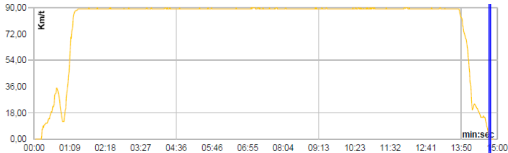
Figure 3: The figure shows that speed in km/h of the HDV 1 EURO VI vehicle during the drive on the highway. The vehicle was driven without a payload. The speed of the vehicle is constant because it drives on the highway.
